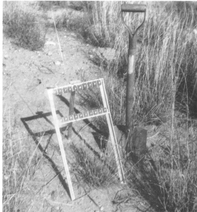
Fig. 1. Point frame and piano wire pin used to sample New Mexico rangelands.
